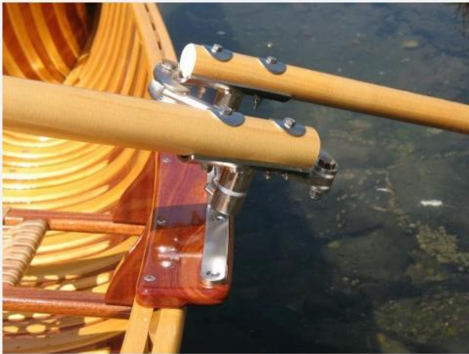
The beam-extending "wings" in use on a canoe.
